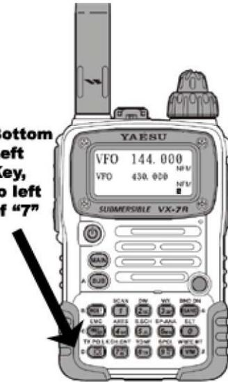
If you hold the key for 2 seconds, it locks the key pad. If you press it just once (or accidentally touch it while holding the radio), it turns wires ON.
